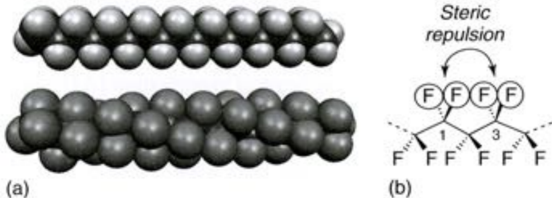
Figure 1.2 The zigzag conformation of octadecane (a) compared with the helical perfluorooctadecane (b), modeled at the PM3 level of theory [39, 40].
